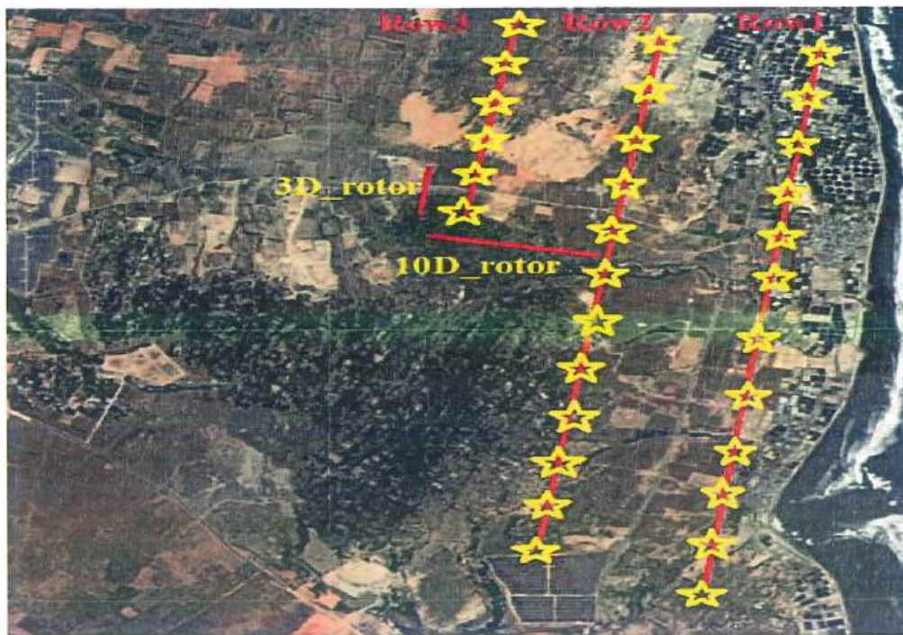
Figure 4.20. Optimum configuration for installing the E103 turbines at the farm
