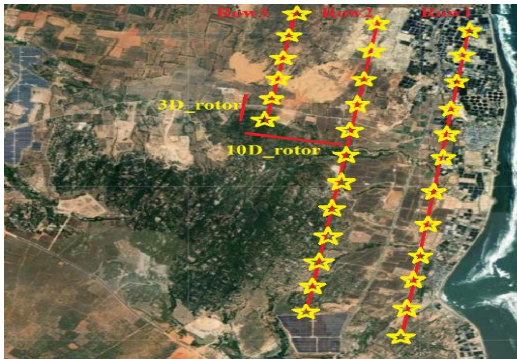
Figure 4.20. Optimum configuration for installing the E103 turbines at the farm area
